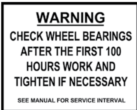
Check the wheel bearings after the first 100 hours work and tighten if necessary.
