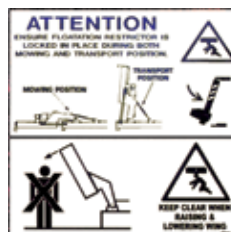
Moving parts hazard
